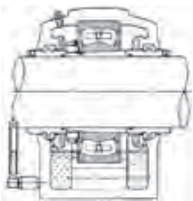
Oil Bath Lubrication: not for high speeds
