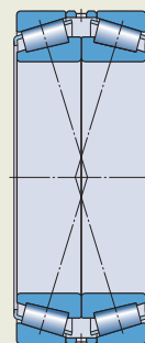
Matched bearings arranged face-to-face
