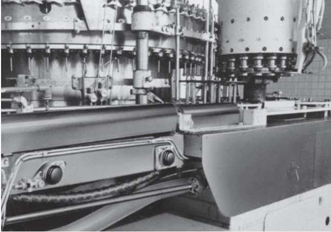
Bottle filling line conveyor
